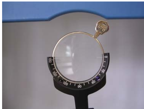
Fig. 6-5 Insert spherical lenses towards the patients eye and cylindrical lenses towards the cupola
